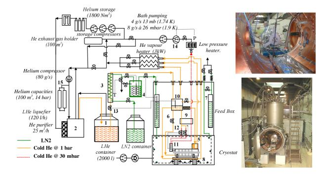
Figure 3: Cryogenic Installation.
