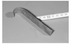
Fig. 5. End spacer machined from copper-aluminum alloy
