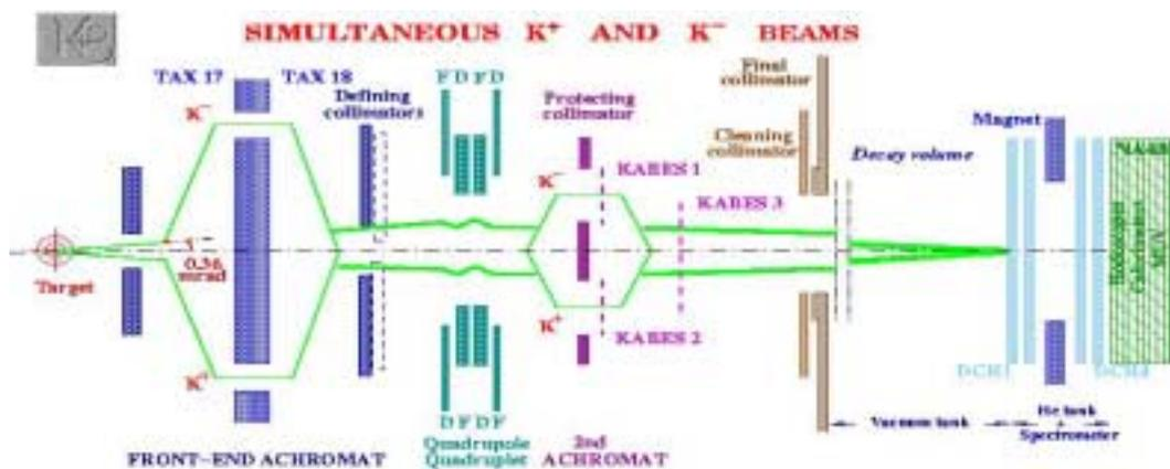
Figure 1: The K12 charged kaon beam line with KABES and  $K^+/K^-$  focusing at the DCH spectrometer.
