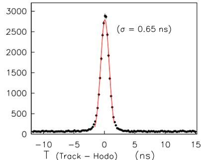
Figure 6: Time resolution of KABES with respect to the trigger hodoscope.
