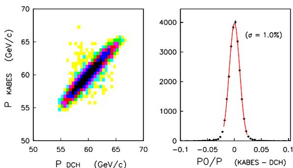
Figure 5: KABES momentum versus DCH spectrometer momentum and their difference.
