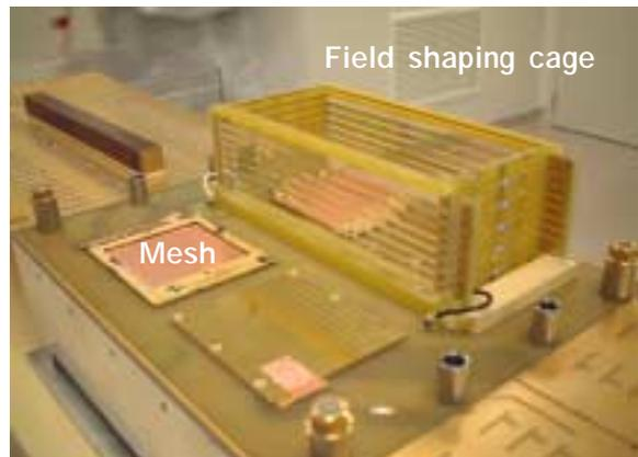
Figure 2: The field cage with aluminum lines and the mesh of the amplification gap.
