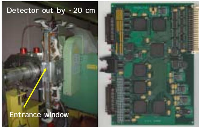
Figure 3: One detector in the K12 beam line (left) and the HPTDC read-out card (right).
