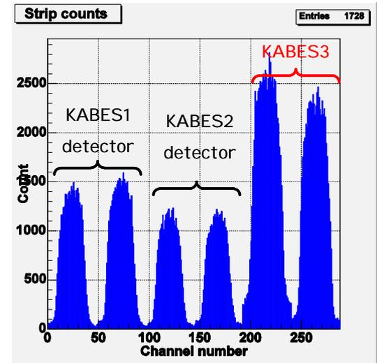
Figure 4: The online display of beam profiles recorded by the three double stations.
