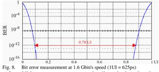
In addition to measurements, the jitter budget has been calculated for all types of communication channels using maximum values of contributed jitter characteristics known for all active devices and passive optical components including splitters and 50 m long fibers. In all cases induced total and deterministic jitters were less than respectively 0.65 UI and 0.41 UI jitter tolerances of RocketIO receivers.
