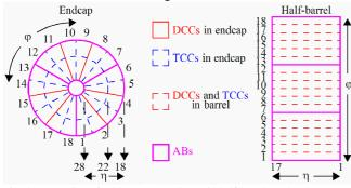
Fig. 5. Mapping of TCCs, DCCs and ABs in half-barrels and endcaps
