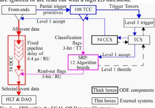
Fig. 3. SRP within the ECAL Off-Detector Electronics
