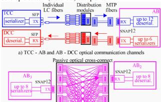
b) Inter-AB optical communications (part of the cross-connect shown) Fig. 7. Organization of the SRP communication channels
