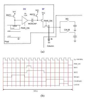
Fig. 1. (a) Schematic of the proposed DC-coupled pixel and, (b) related timing (clocking stimuli) with  $f_{CK}$ =100 MHz. RD, CALIB and LATCH signals are used by the column readout circuitry.
