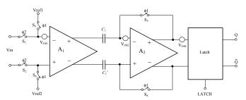
Fig. 4. Bloc diagram of the offset compensated comparator.
