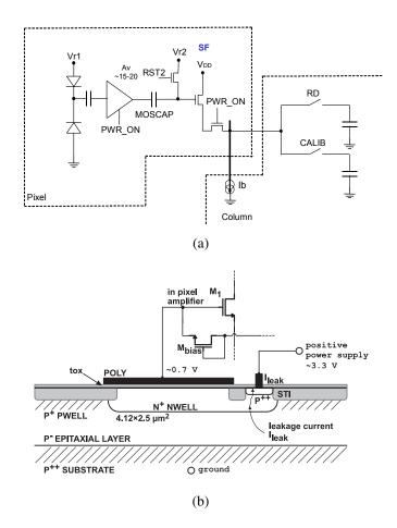
Fig. 2. a) Schematic of the proposed AC-coupled pixel, and b) principle of the direct AC coupling of the auto-reverse polarized charge sensitive element and the amplifier.
