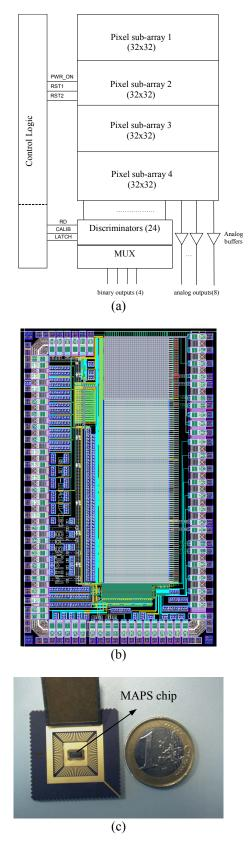
Fig. 3. a) Block diagram, b) layout and c) photography of the realized prototype chip.
