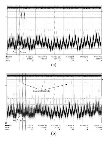
Fig. 6. Output analog signal from 32 pixels of a column recorded on a scope (20 mV/div.) a) with few small-amplitude hits, and b) with multiple high-amplitude hits.
