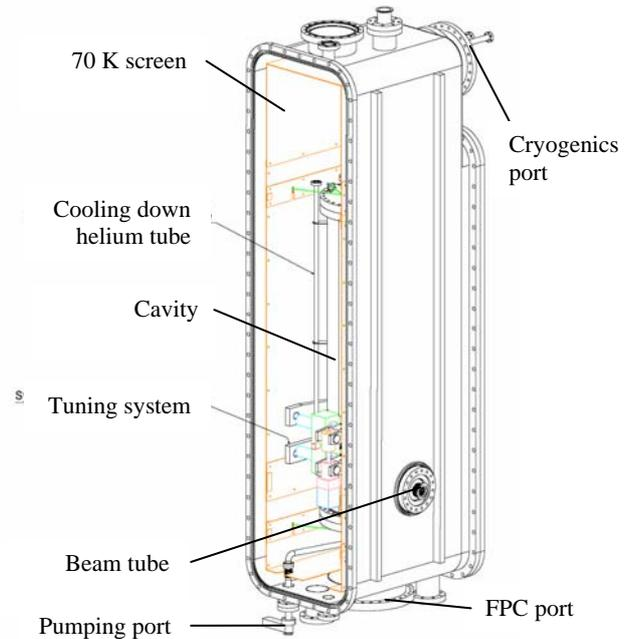
Figure 5: Cryomodule general scheme.
