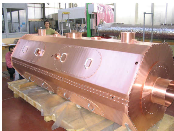
Figure 2: Copper thermal shield with 8 dismountable access doors.
