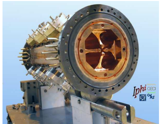
Figure 4 : the first RFQ section viewed from the beam entrance side
