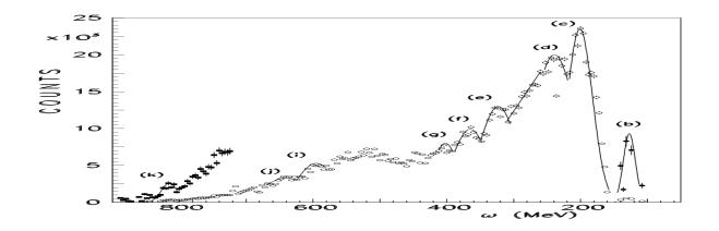
Figure 1: Spectra of the  $p(\alpha, \alpha')X$  reaction studied at SPES4 (Saturne) with  $T_{\alpha}=4.2$  GeV and  $\theta=0.8^{0}$  [2].
