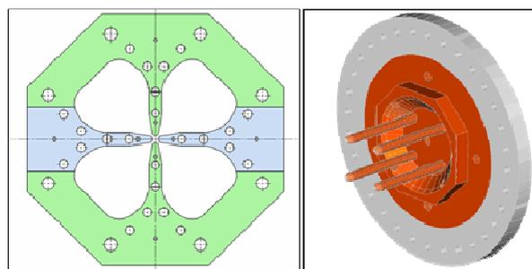
FIGURE 2. The four brazing parts and a coupling plate with the dipole fingers.
