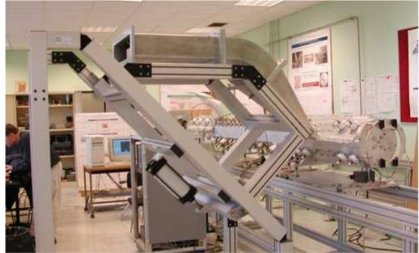
**FIGURE 5.** View of the 6-m long RFQ cold model
