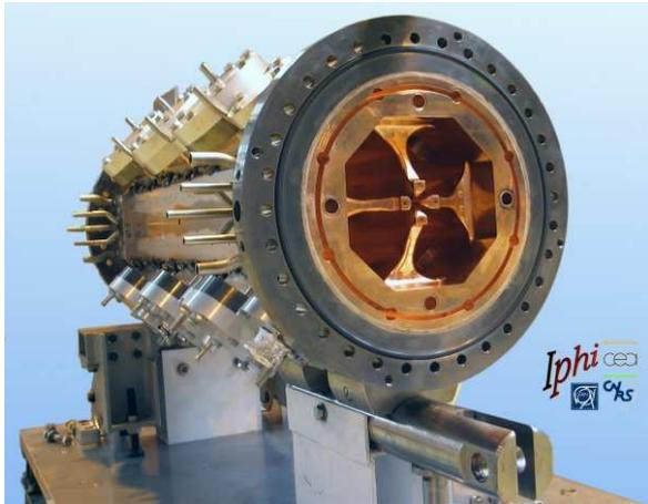
**FIGURE 3.** the first RFQ section viewed from the beam entrance side.
