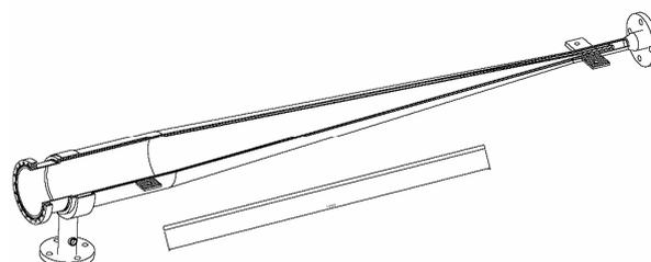
FIGURE 8. 3D view of the conical beam dump showing the water inlet and outlet.
