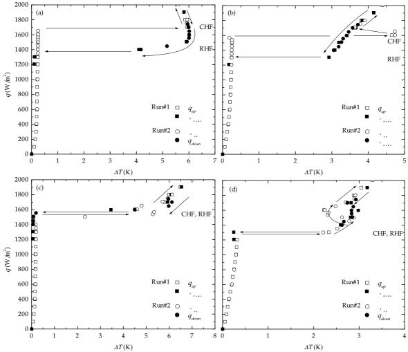
**FIGURE 3.** Boiling curves for the temperature sensor at different height: (a) L=0.3 m or L/D = 21.4, (b) L=0.6 m or L/D = 42.8, (c) L=0.9 m or L/D = 64.3 and (d) L=1.2 m or L/D=85.7.
