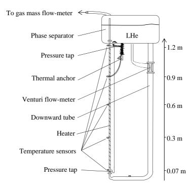
FIGURE 1. Schematic of the test section.
