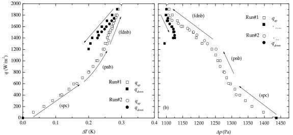
**FIGURE 2.** (a) Boiling curve for the temperature sensor at a height of L=0.07 m, L/D=5 - (b) Heat flux as a function of the total pressure variation of the tube,  $\Delta p$ .
