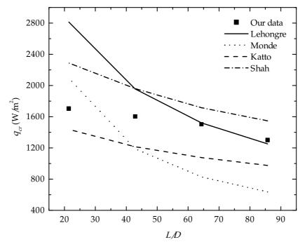
**FIGURE 5.** Comparison between experimental data and the different correlations as a function of L/D.
