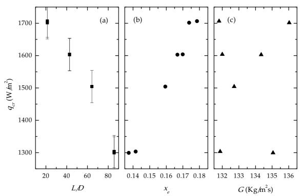
**FIGURE 4.** Critical heat flux  $q_{cr}$  (a), the vapor quality at the exit,  $x_e$  (b) and the total mass flux G (c) as a function of the L/D ratio
