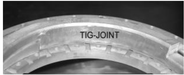
Fig. 8. A TIG-joint round sample in the “shaking hands” configuration for measurements in Ma.Ri.S.A.
