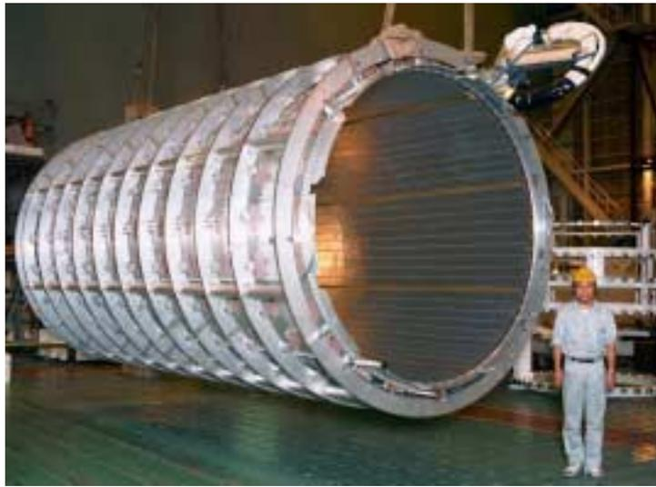
Fig 6. The ATLAS Central Solenoid
