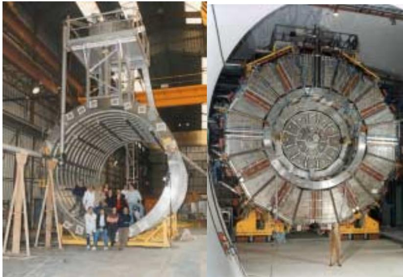
Fig 3. The Aleph solenoid alone (left) and inside the detector (right)
