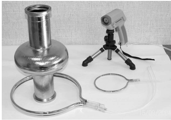
FIGURE 14. 1.3 GHz cavity, IR heaters and thermal sensor for “fast / air baking” in clean room.
