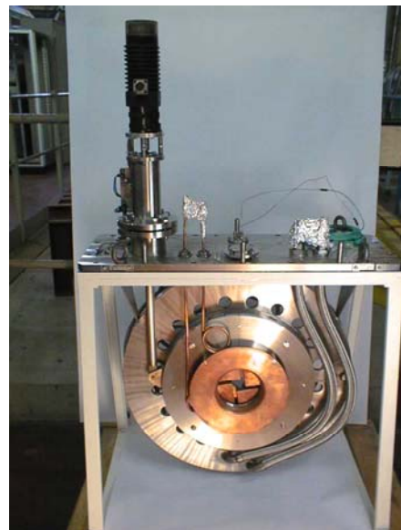
Figure 3-32 – Example of a water-cooled iris.
