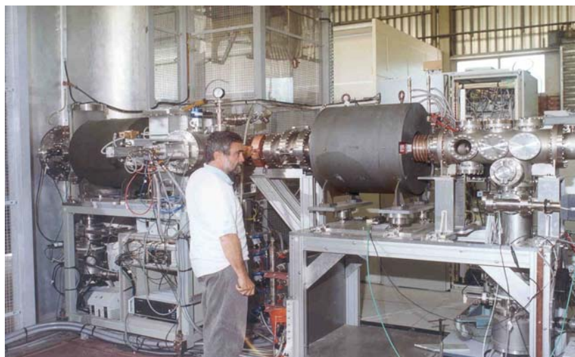
Figure 3-8 – The SILHI LEPT installed at CEA Saclay.
