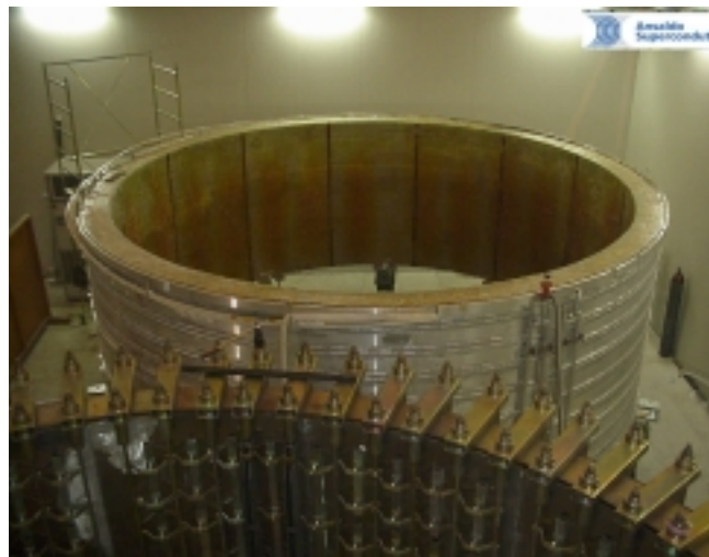
Fig. 9. CB-2 after impregnation (back). CB-1 in preparation for impregnation (front).
