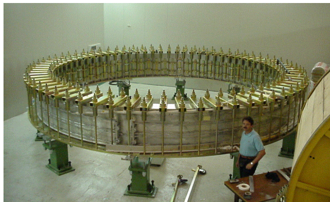
Fig. 4. The prototype, coil after winding, ready for impregnation and equipped with clamps.
