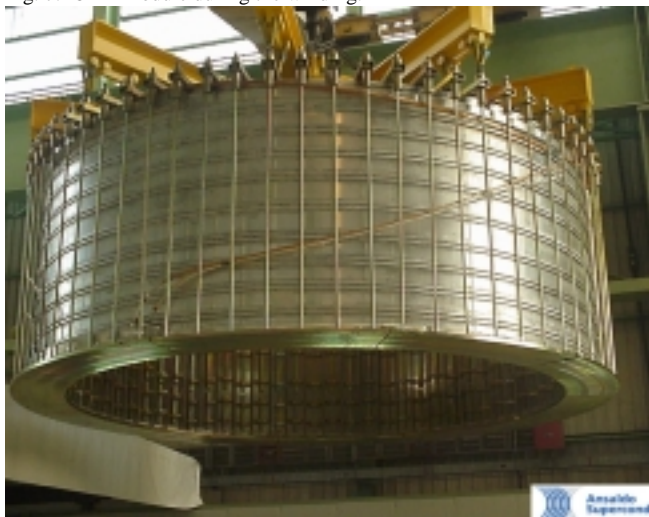
Fig. 8. CB-2 module ready for vacuum impregnation under vacuum. The coil is axially pressed at 1.2 MPa using 140 stainless steel tie-rods. Belleville washers are placed on both upper and lower flanges in order to keep the axial load in any stage of the impregnation process.
