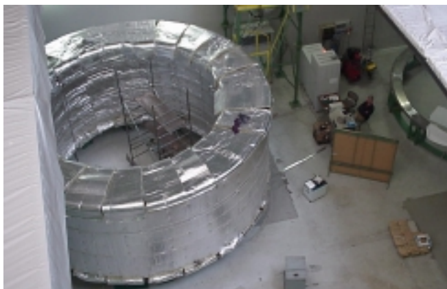
Fig. 5. Top view of the vacuum vessel during prototype impregnation.
