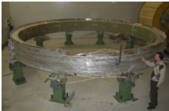
Fig. 6. The prototype coil as extracted from the mold after impregnation.
