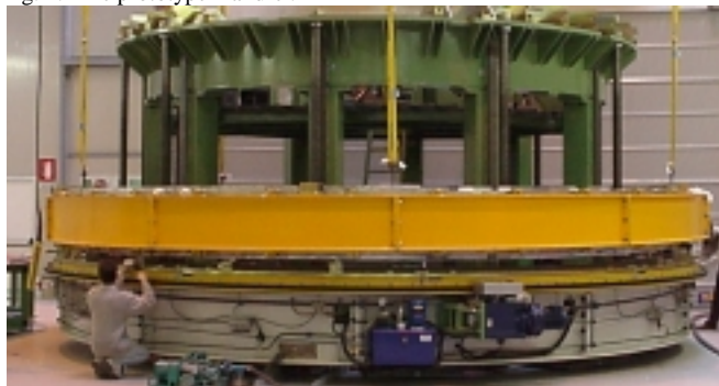
Fig. 2. The prototype mandrel with the outer reinforced ring is mounted onto the winding table.
