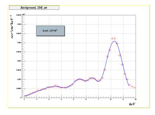
Fig. 5. Micromegas detector background data after cuts. The level achieved is  $2.0*10^{-5}$  events/keV/cm<sup>2</sup>/sec between 1-10 keV.
