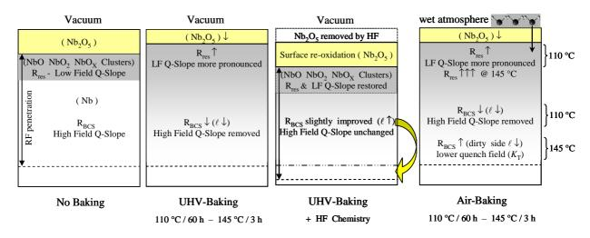
Figure 6: Sketches of Nb surface (layer scale is not respected) summarising experimental changes of  $R_{BCS}$ ,  $R_{res}$ , high and low field Q-slopes after baking and HF cavity treatments.
