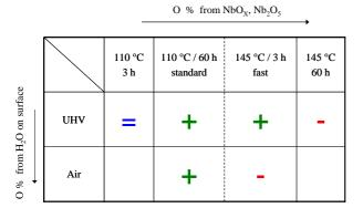
Figure 5: Overview on the different baking experiments with improvement (+), degradation (-) or without modification (=) of the  $Q_0$  ( $E_{acc}$ ) curve.
