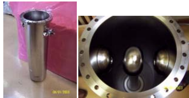
Figure 3: Cavity prototype (outer and internal views).
