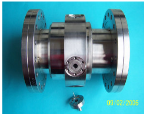
FIGURE 3. Drawing and photo of the modified BPM cavity.
