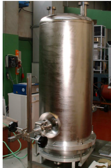
Figure 8: \beta=0.12 QWR during frequency adjustment
