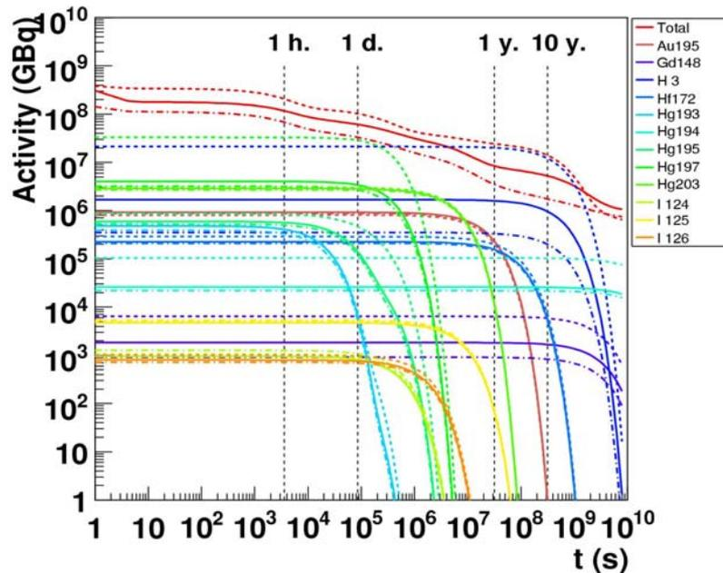
**Figure 10** : Radioactivity estimates as a function of cooling time using ISABEL-ABLA (solid line), CEM2k (dashed line) and INCL4-ABLA (dashed-dotted line) models.
