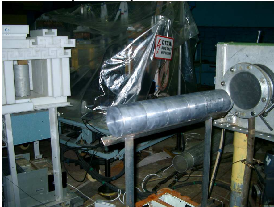
Figure 1: A photo of the experimental setup to measure DNs from p(1GeV)+Pb with the proton beam line (on the right), the Pb target (in the center) and He-3 counter (on the left).
