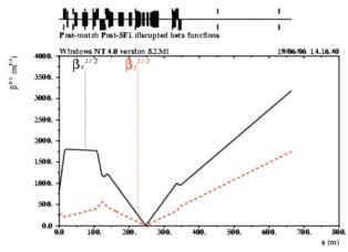
Figure 1: The matched linear optics for the 500 GeV CM extraction line, using the optimised NbTi final doublet layout.
