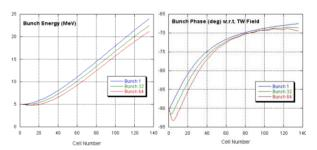
Figure 3: Bunch energy and phase at the exit of compression section at full current.
