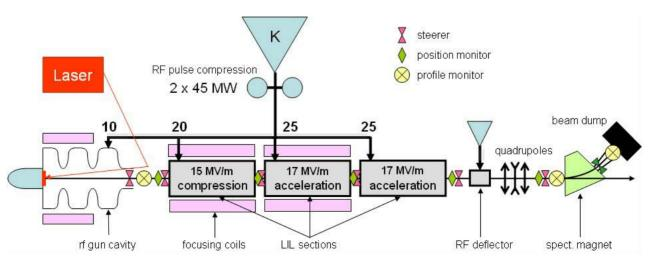
Figure 1: Schematic layout of the probe beam linac (Califes).
