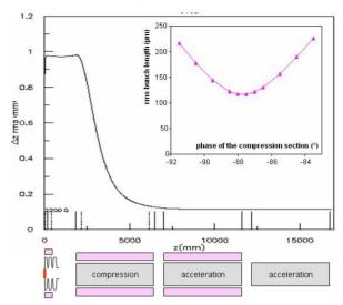
Figure 2: rms bunch length along the linac and sensitivity to the RF phase (box).
