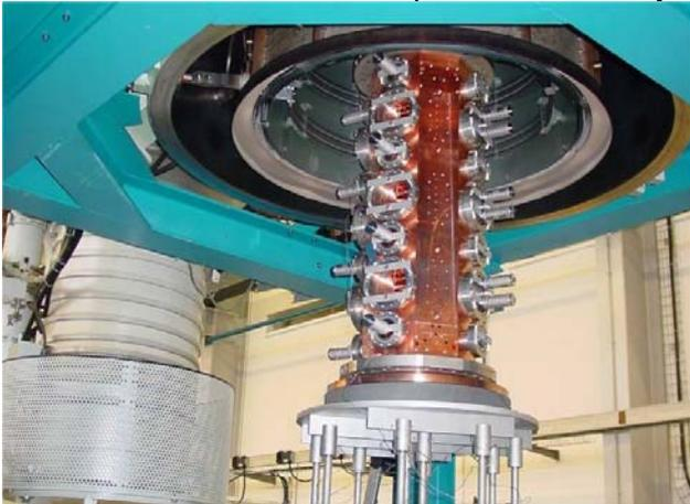
Figure 3 : the second section of the IPHI RFQ entering the brazing furnace.
