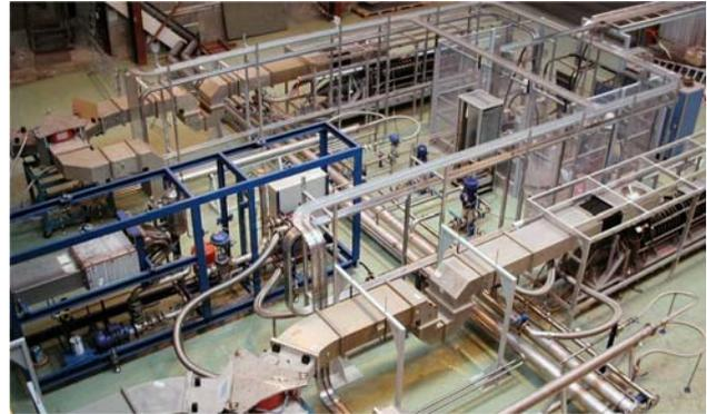
Figure 4 : View of the RF power system showing the two klystron lines, the circulators and the 1.4 MW, salt water load.
