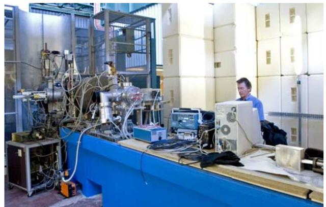
Figure 2 : view of the source and the LEBT at Saclay. A part of the LEBT is located on the RFQ concrete support.
