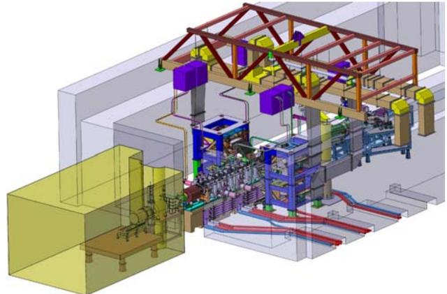
Figure 1 : 3D view representing the final arrangement of the IPHI injector.
