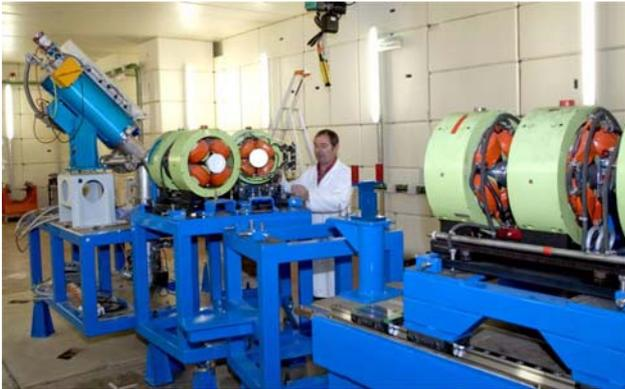
Figure 6 : Installation in progress of the diagnostics line with the wire-scanner on the left.
