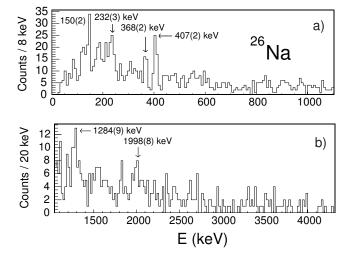
FIG. 11: Low-energy (a) and high-energy (b) part of the  $\gamma$  spectrum of  $^{26}$ Na. The spectrum is Doppler corrected with a velocity  $\beta{=}0.095$ . The neutron separation energy of  $^{26}$ Na is  $S_n{=}5.576(6)$  MeV [38].
