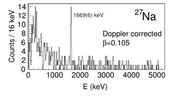
FIG. 10: Doppler-corrected  $\gamma$  spectrum of  $^{27}$ Na. The neutron separation energy of  $^{27}$ Na is  $S_n{=}6.726(7)$  MeV [38].
