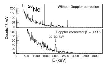
FIG. 3:  $\gamma$ -ray spectrum of <sup>26</sup>Ne without (top) and with (bottom) Doppler correction. Sharp lines in the uncorrected Doppler spectrum are due to well known transitions from room background.
