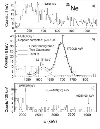
FIG. 7:  $\gamma$ -spectrum of <sup>25</sup>Ne. (a) The low-energy part of the spectrum shows a 320 keV transition, present in all angular rings. (b) Zoom of the 1700 keV region: the result of the fit for two transitions at 1621 keV and 1700 keV is shown. (c) High-energy region: the low background allows for sensitivity to transitions with low statistics.
