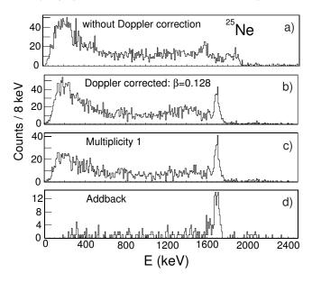
FIG. 6:  $\gamma$ -ray spectra of <sup>25</sup>Ne: without Doppler correction (a), Doppler corrected with a velocity  $\beta$ =0.128 (b), multiplicity 1 events only (c), addback events (d).
