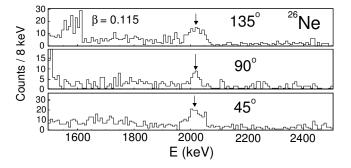
FIG. 4: Doppler corrected de-excitation  $\gamma$ -ray spectrum of  $^{26}\mathrm{Ne}$  for the three detection angles : 45° (bottom), 90° (middle), and 135° (top). The structure at  $\sim \! 1600$  keV in the 135° spectrum comes from the Doppler correction of the 1460 keV background transition.
