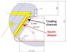
Figure 2: IPHI vane end profile and cooling channel.
