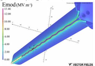
Figure 4: <sup>1</sup>/<sub>4</sub> of IPHI 6<sup>th</sup> segment simulation with SOPRANO.
