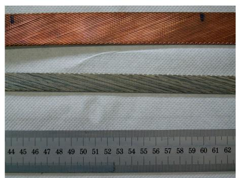
Figure 3: Photo of a 40-strand Rutherford-type cable produced by LBNL with SMI/NED wire (top) compared to a 28-strand LHC inner layer cable (bottom).
