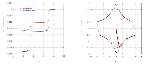
Figure 2: Magnetization measurements on SMI/NED wire: (a) as a function of temperature (left) and (b) as a function of field (right; courtesy of P. Fabbricatore and M. Greco, INFN-Genoa, C. Ferdeghini, INFM-Genoa and U. Gambardella, INFN-Frascati).
