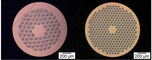
Figure 1. Cross-sectional views of wires developed within the framework of the CARE/NED activity: (a) Internal Tin wire produced by Alstom/MSA (left) and (b) Powder-In-Tube wire developed by SMI (right).
