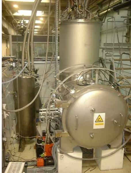
Figure 1: CryHoLab, a horizontal cryostat located at CEA Saclay
