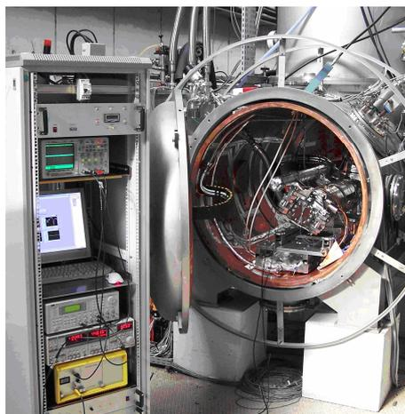
Figure 15: Integrated instrumentation for transfer function measurement
