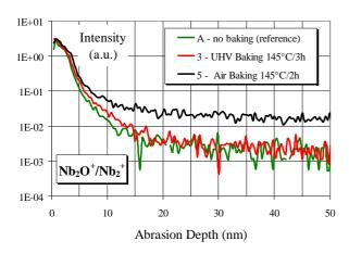
Figure 4: Interstitial oxygen profiles by SIMS analyses on niobium samples before and after fast baking (under vacuum and air atmosphere) [8].
