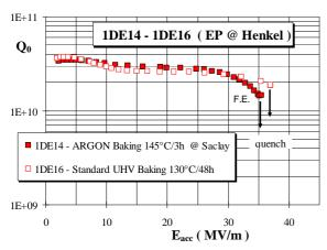
Figure 7: Comparison between "Standard UHV" and "Fast Argon" Baking.
