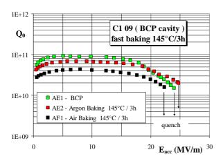
Figure 3: Baking effect (145°C for 3 hours) after BCP on cavity filled with argon (red data) and open to the room atmosphere (black data) [7].
