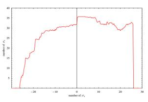
Figure 1: Dynamic aperture for 1000 turns without a defect in the dipoles. The horizontal and vertical emittances are taken equal to  $0.22 \pi$  mm.mrad
