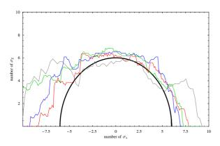
Figure 4: Dynamic aperture at 1000 turns for different working points after optimization (in gray for A before optimization, in red after, in blue for B and in green for C)
