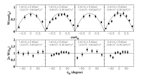
FIG. 5: Decay angular distributions of the  $\phi$ -meson in the helicity frame. The inner error bars shown are statistical uncertainty only, while the outer error bars are the sum of statistical and systematic uncertainties in quadrature. Solid curves are the predictions from helicity conservation.
