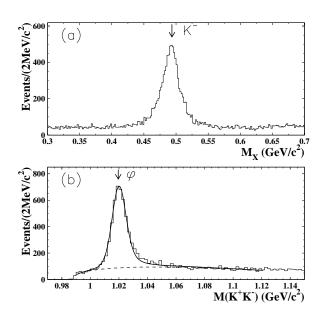
FIG. 2: (a) Missing mass distribution of the reaction  $\gamma d \rightarrow dK^+ X$  for events near the  $\phi$ -meson mass (0.98 <  $M(K^+K^-) < 1.12 \text{ GeV/c}^2$ ). (b) Invariant mass distribution for the  $K^+K^-$  pair after the selection of the missing  $K^-$ . The solid curve is a fit to the data. The dashed curve shows the contribution from background.
