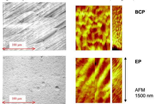
**FIGURE 2.** Surface aspect of BCP and EP on a (110) monocrystals at different scales (left: optical, right, tunneling microscopy). At very low scale, the roughness is alike with both surface treatments, whereas at the micron scale, we can clearly observe faceting due to the preferential etching with BCP
