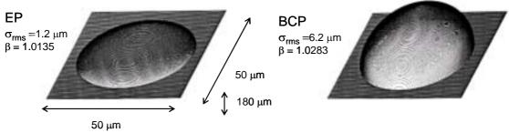
**FIGURE 2.** Equivalent conformal ellipsoids for EP and BCP polycrystalline surfaces, along with the measured roughness ( $\sigma$ ) and the field enhancement factor ( $\beta$ , mean value). ~10 grains are scanned.
