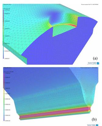
Figure 2: One-quarter of RFQ cross section with 2 half slugs meshed with I-DEAS and solved with SOPRANO (a) Magnetic field, (b) Electric field
