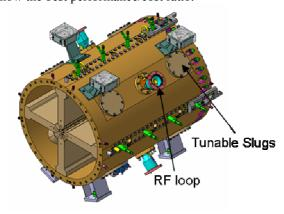
Figure 1: Location of tuner slugs and loop port in one 1-meter long RFQ module (final design).
