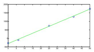
Figure 4: 3D frequency shift (kHz) vs. tuner position even part h<sub>OO0</sub> (mm). 0 kHz reference: 2D simulation.
