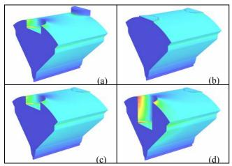
Figure 3: SOPRANO models corresponding to different tuner positions [#1,#2]: (a) [-30,+50], (b) [+0,+0], (c) [+50,+0], (d) [+130,+0].
