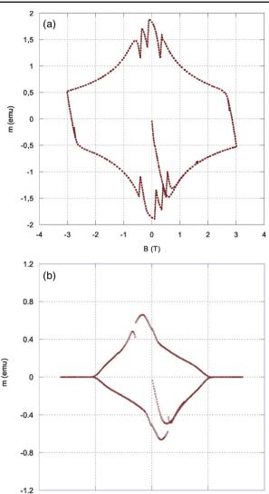
**Figure 2.** The dc magnetic moment as a function of the magnetic field (transverse to the wire) measured in 5 mm long samples of NED wire at 4.5 K. In (a) the measurement on a reacted wire is shown. In (b) one can see the measurements on an unreacted wire (so only Nb properties affect the magnetic moment).
