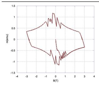
**Figure 4.** The dc magnetic moment as a function of the magnetic field (transverse to the wire) measured in a sample of a PIT wire composed of 192 filaments at 4.5 K. With respect to the case of figure 1, the unreacted region is larger ( $\chi = 1.48$ ).
