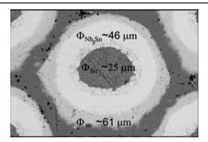
**Figure 1.** SEM image showing the cross section of a single filament of a PIT wire developed in the framework of the NED project. The approximate dimensions of each filament phase (Sn, Nb and Nb<sub>3</sub>Sn) immersed in a Cu matrix are reported too.
