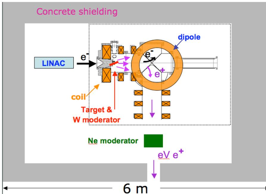
**Figure 2** Schematic layout of the planned positron source.
