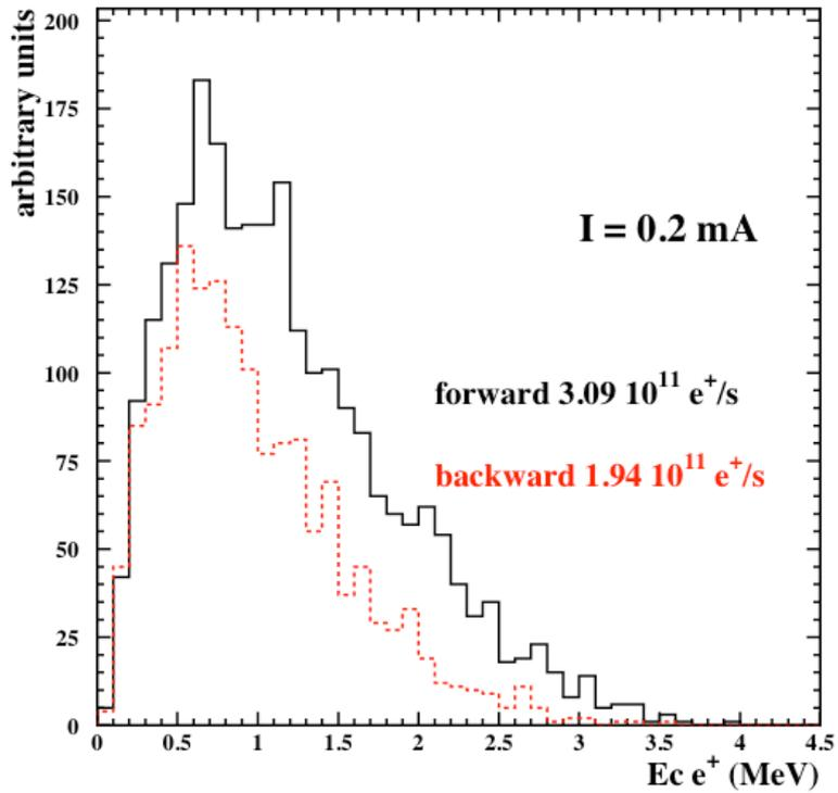
**Figure 1** Kinetic energy spectrum of the produced positrons in 100 keV bins, for 6 MeV electron energy. The integral forward and backward emitted rates are shown.
