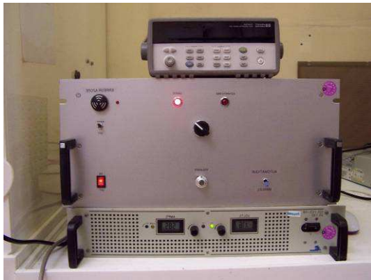
Figure 14a : Central unit located on top , rack with electronics located in the middle and power supply located on bottom of the setup view.
