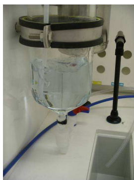
Figure 11a : Scrubber filled with BTB.
