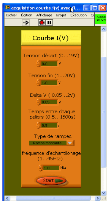
Figure 15a : Parameters chosen for I(V) curves plotting: voltage boundaries, frequency, scan rate, possible reverse scan.
