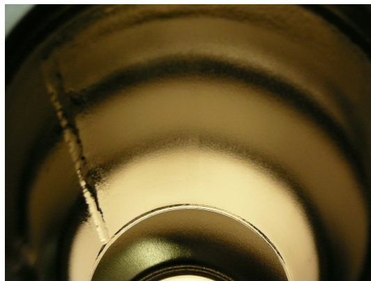
Figure 28: Internal surface of 1C21 cavity after 130 \mu\text{m} removal with EP at 5 volts.
