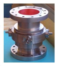
Figure 4: Re-entrant cavity BPM
