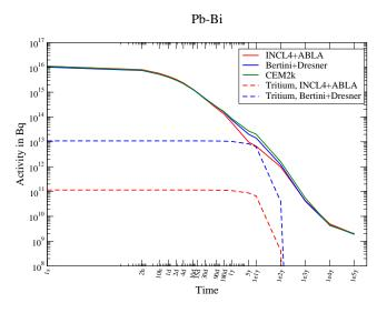
**Figure 4:** Total activity of the LBE as a function of cooling time after 123 days of irradiation with 575 MeV protons at 0.947 mA using different models. Dashed curves show the contribution of tritium to the total activity.
