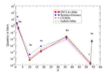
Figure 8: Quantity of gaseous elements produced in LBE using several models. These calculations were done after 123 days of irradiation with 575 MeV protons at 0.947 mA.
