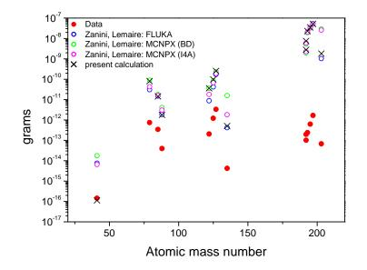
Figure 12: Comparison of different calculations with measurements of volatile elements released in the expansion volume of the LBE among which INCL4-ABLA and Bertini-Dresner denoted respectively MCNPX (I4A) and MCNPX (BD) in the legend.
