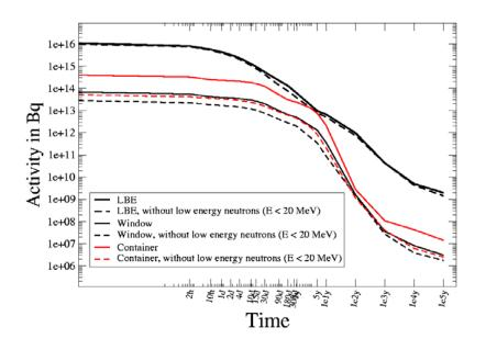
Figure 3: Activity of the LBE, container and window. Full activities are in solid lines and activities without low energy neutron (E < 20 MeV) contribution are in dashed lines. The calculation is done using INCL4-ABLA.
