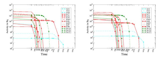
Figure 11: Main contributors to the activity in LBE coming from gaseous elements as a function of cooling time using INCL4-ABLA (left) and Bertini-Dresner (right).
