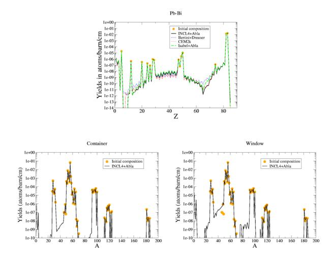
**Figure 13:** Concentration of elements after 123 days of irradiation by 575 MeV protons at 0.947 mA Charge distribution (top) for the LBE with the four models and mass distribution for container and window (respectively bottom left and right) with INCL4-ABLA only. Initial compositions are represented as full orange dots.
