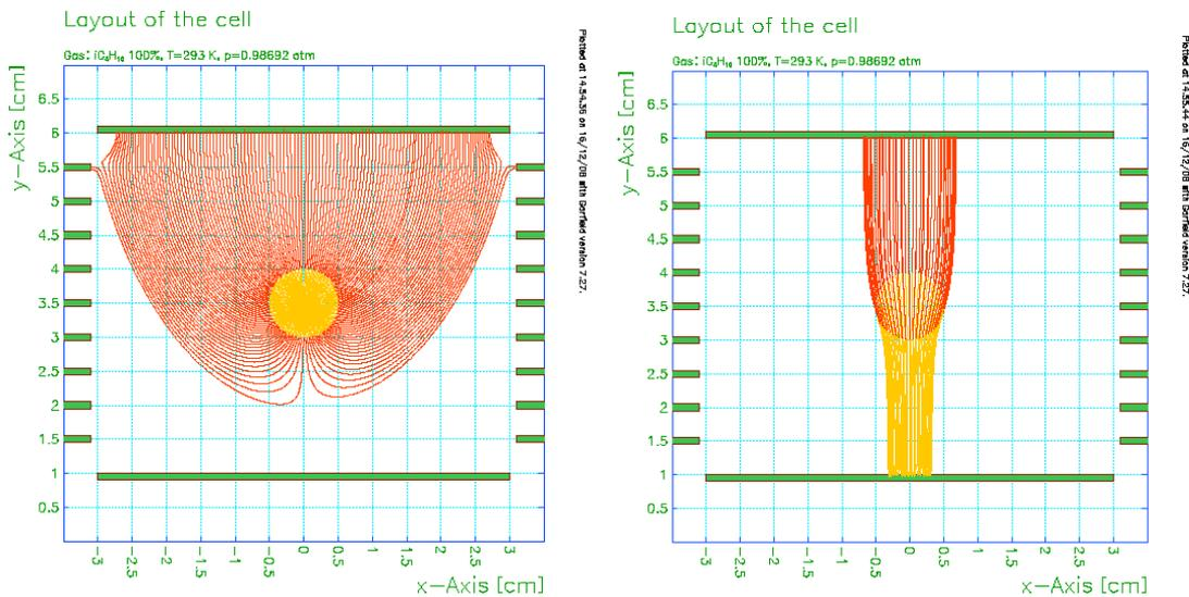
Fig. 5: Electric field lines at -200 V on the left and -2000 V on the right with the ions in red and the electrons in yellow.
