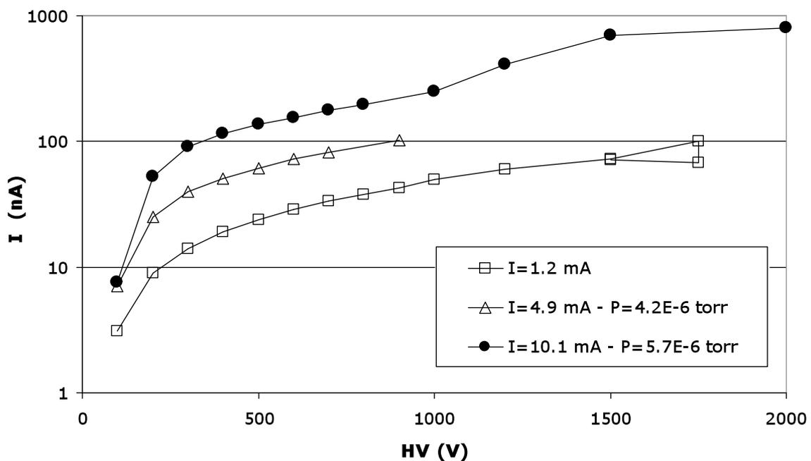
**Fig. 6:** Current read on 2 central strips for a positive polarisation.
