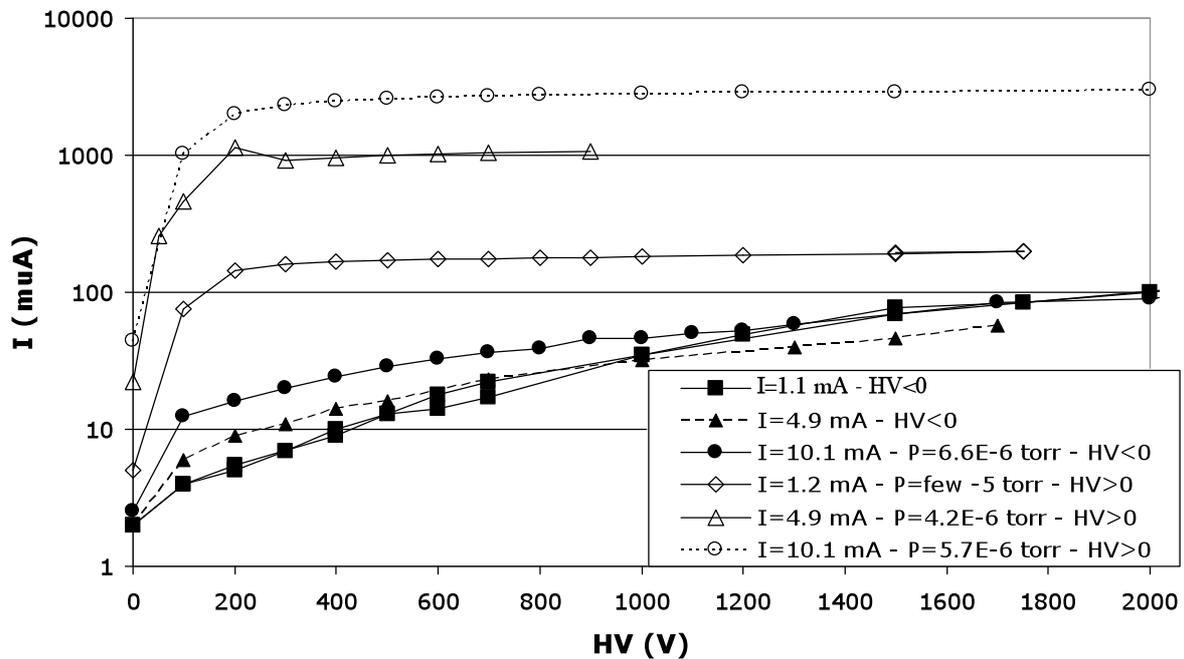
**Fig. 3:** Absolute value of the current read on the high voltage module in positive and negative potentials and for different beam intensities.
