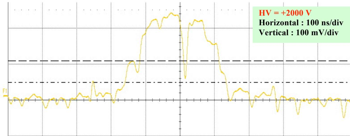
**Fig. 8:** Oscilloscope beam profiles.
