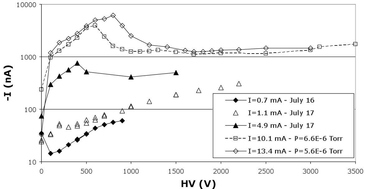
**Fig. 7:** Current read on 2 central strips for a negative polarisation.
