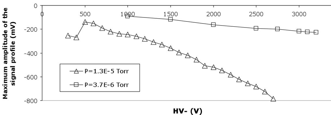
**Fig. 9:** Amplitude of two beam profiles at different pressures as a function of the drift voltage.
