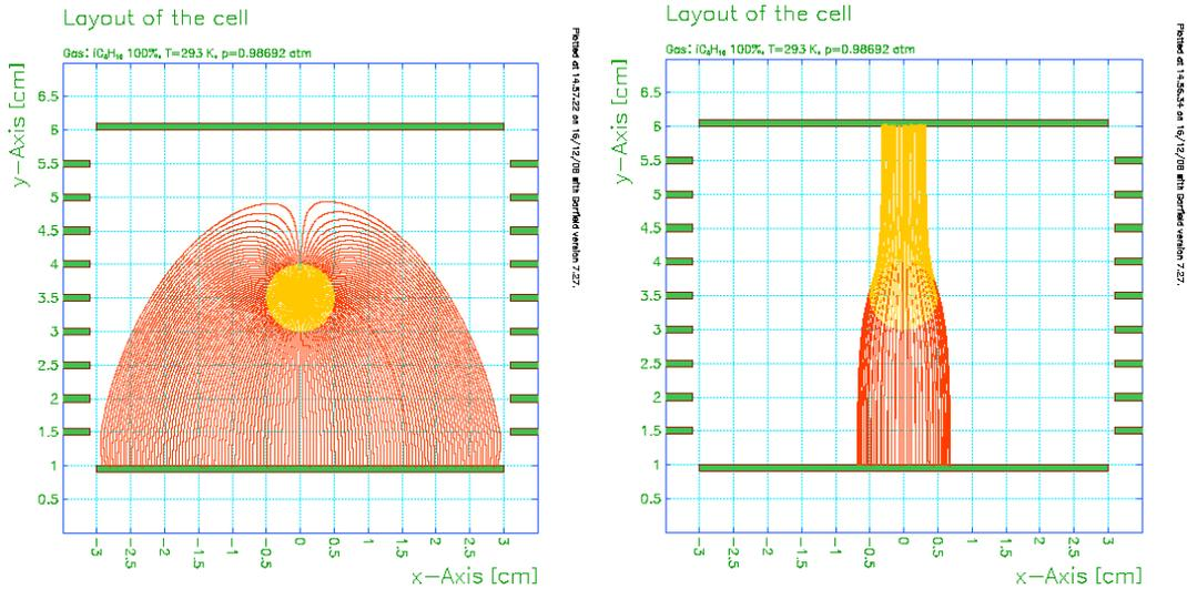
Fig. 4: Electric field lines at +200 V on the left and +2000 V on the right with the ions in red and the electrons in yellow.
