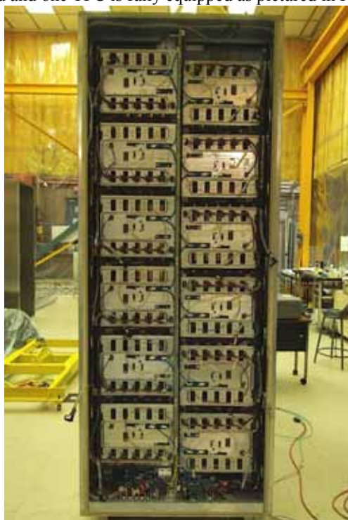
Fig. 7. One of the two end plates of a fully equipped TPC.
