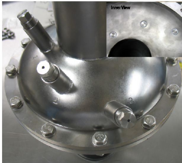
Fig.1: Demountable cavity for BEP study. and iris, and close to iris. The Nb buttons are processed together with the cavity and then they can be removed for various analyses. For consistency, the buttons were made from the same Nb batch. The buttons are also electrically insulated from the cell to allow the measurements of I-V curves at the three locations. After the fabrication, this demountable cavity was shipped to PKU for doing experiments.
