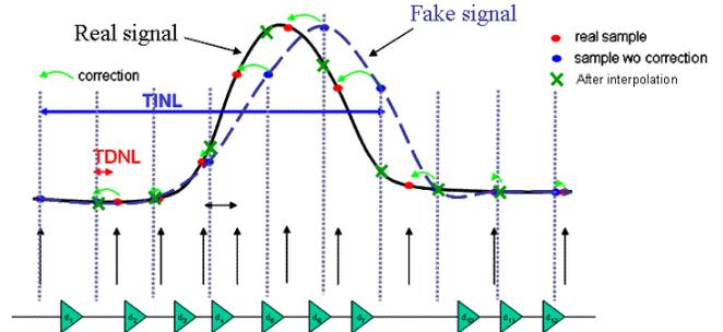
Figure 8: effect of Fixed Pattern Time Distribution on signal sampling.
