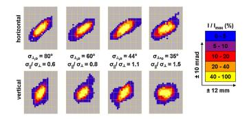
FIG. 3 (color online). Phase space distributions measured at the DTL exit for zero current phase advances  $\sigma_{\perp,o}$  of 35°, 44°, 60°, and 80°. Upper panels: horizontal; lower panels: vertical. The scale is  $\pm 12$  mm and  $\pm 10$  mrad. Fractional intensities refer to the phase space element including the highest intensity.
