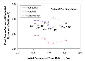
FIG. 7 (color online). Simulated beam currents within the initial rms emittance at the DTL exit as a function of the initial ratio of depressed longitudinal and transverse tune  $\sigma_{\parallel}/\sigma_{\perp}$ .
