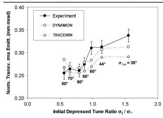
FIG. 4. Mean of horizontal and vertical rms emittance at the DTL exit as a function of the initial ratio of depressed longitudinal and transverse tune  $\eta = \sigma_{\parallel}/\sigma_{\perp}$ .
