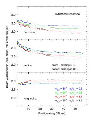
FIG. 6 (color online). Beam current within the initial rms emittance as a function of position using the DYNAMION code. Solid lines correspond to the DTL used for the measurements, while dotted lines indicate results corresponding to a virtually prolonged DTL.
