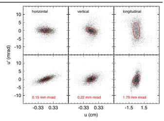
FIG. 5 (color online). Phase space distributions (u, u' referring to the horizontal/left, vertical/center, and longitudinal/right coordinate) corresponding to the  $\sigma_{\perp,o} = 60^{\circ}$  case from simulations with the DYNAMION code. Top: DTL entrance; bottom: DTL exit.
