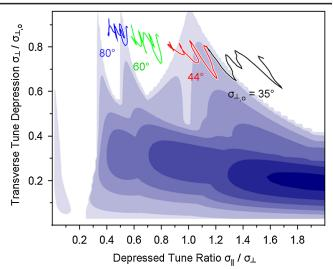
FIG. 2 (color online). Example of Hofmann stability chart for emittance ratio 10 and simulated paths of the depressed tunes for transverse zero current phase advances  $\sigma_{\perp,o}$  of 35°, 44°, 60°, and 80°.
