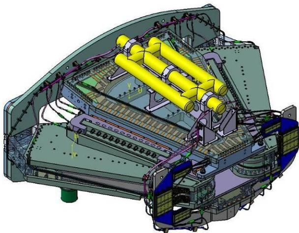
Fig. 3. The cold mass assembly including coils, coil-casings, structural linking components and other non-structural components.
