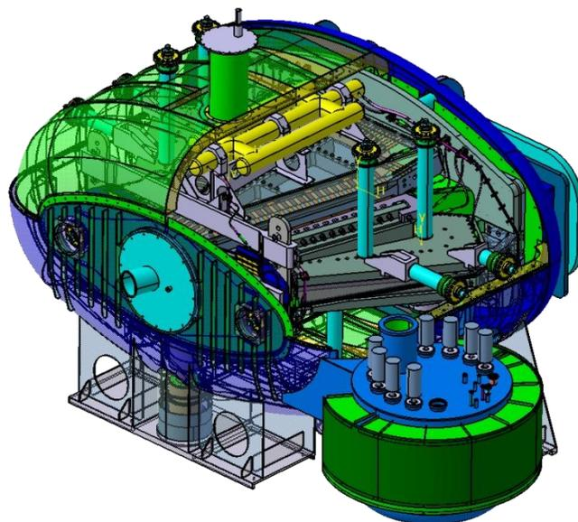
Fig. 2. Main components of the cryostat: the cold mass (grey) with the thermosiphon cooling reservoir (yellow) inside the cryostat (blue) with thermal screen (light green) and satellite (blue & green).
