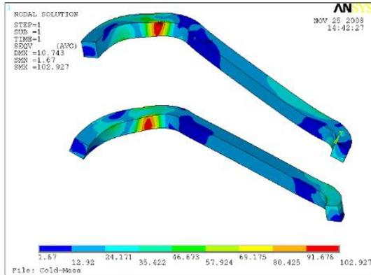
Fig. 6. In the main coil, the thermal stresses are generally less than 50 MPa except some local stress concentrations around 102 MPa.
