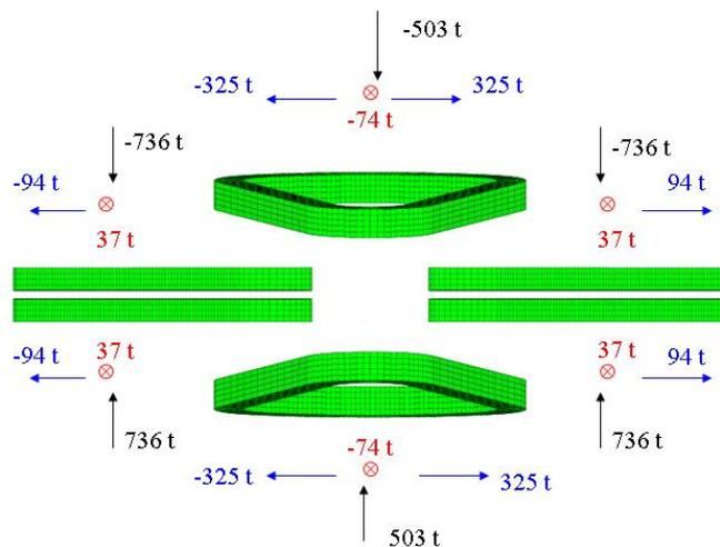
Fig. 4. The resultant magnetic forces of each coil and the relative forces between the 6 coils.
