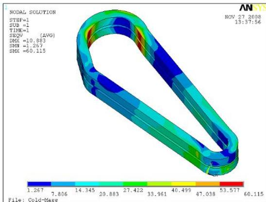
Fig. 7. In the lateral coil, the thermal stresses are all less than 60 MPa.
