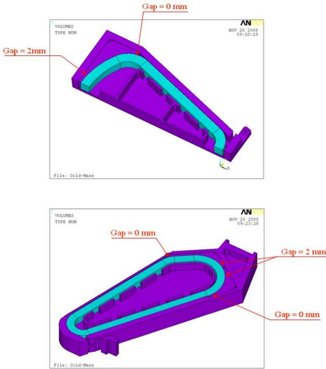
Fig. 5. The necessary initial gaps between coil and wedges during warm assembly phase (upper view: main coil, lower view: lateral coil).
