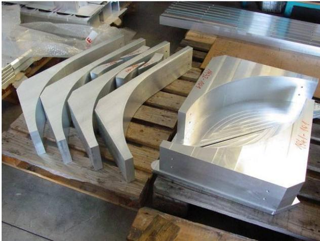
Fig. 11. Wedges after pre-machining (courtesy of ASG Superconductors S.p.A., Genova, Italy)
