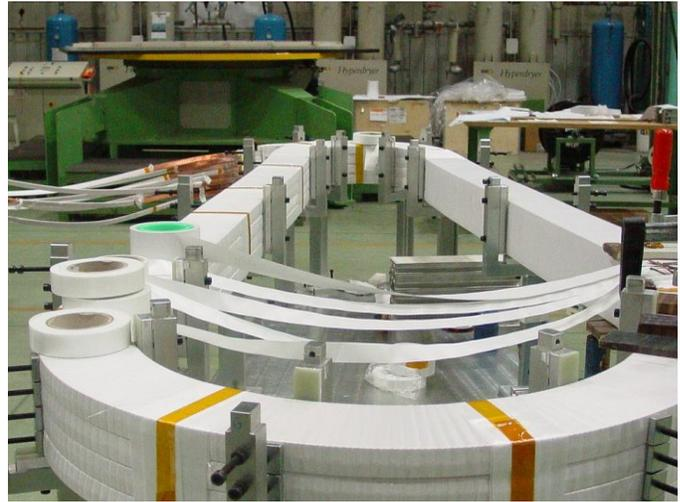
Fig. 12. The double-pancakes are stacked on a special tool, for receiving fiberglass ground insulation before impregnation (courtesy of ASG Superconductors S.p.A., Genova, Italy)
