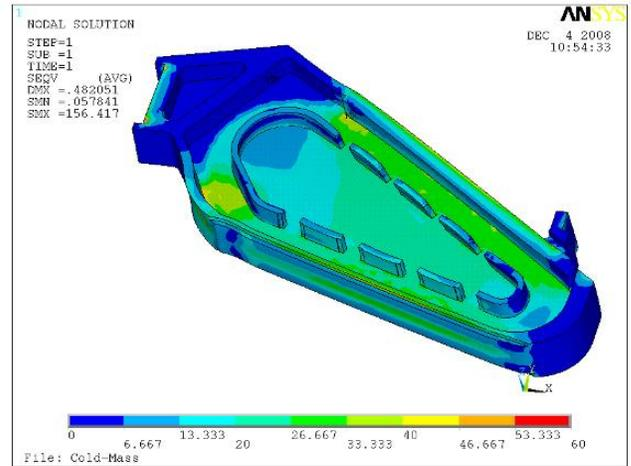
Fig. 9. The Von Mises stress [MPa] distribution in the lateral coil during magnet energizing.
