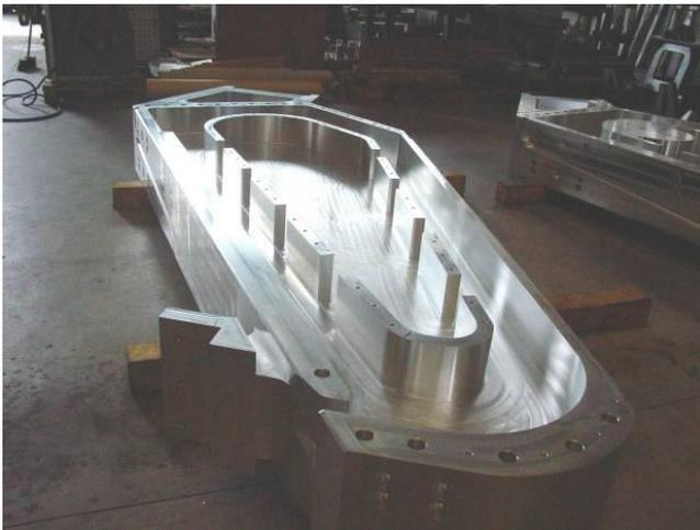
Fig. 10. Lateral coil casing after pre-machining (courtesy of ASG Superconductors S.p.A., Genova, Italy)
