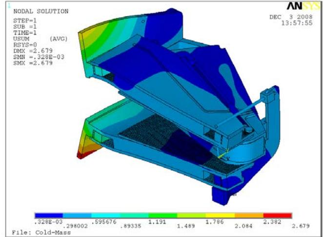
Fig. 8. Deformation contour [mm] of the cold mass structure during magnet energizing.
