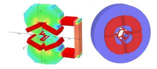
Figure 2. Left: Opened yoke multipole [CEA Saclay Irfu/SACM] and Right: Closed yoke multipole [GANIL]
