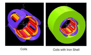
Figure 3. Superconducting multipole [Argonne National Lab.]
