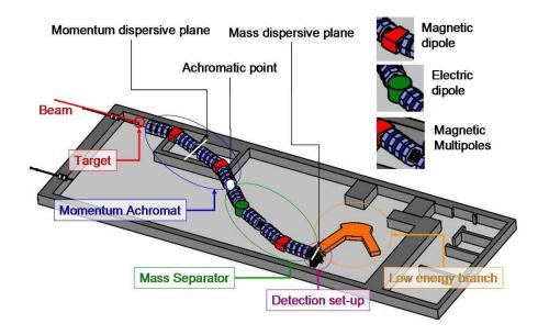
Figure 1. Basic design of the Super Separator Spectrometer.
