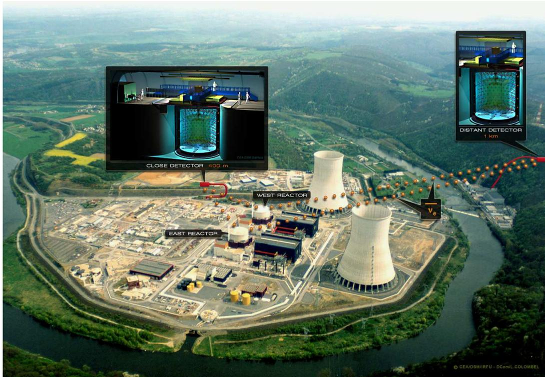
Figure 3.7: Overview of the Double Chooz experimental site. The two underground laboratories are located at the end of the two 150 m tunnels (in red).
