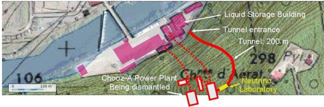
Figure 3.9: Double Chooz far neutrino laboratory, located in a tunnel of the old Chooz-A power station, at distance 1.05 km in average from the Chooz-B nuclear cores. The laboratory is shielded by 300 m.w.e. of rock. The liquid Storage building, also named liquid Storage area is dedicated to the storage of all four liquids prior to detector filling.
