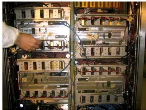
Figure 5.13: Four MicroMegas modules with their electronics installed on the TPC.
