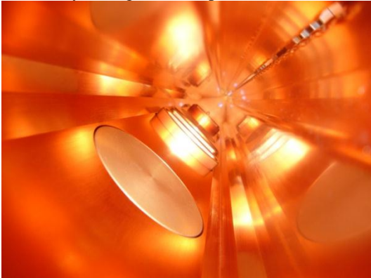
Figure 2: Trying different penetration depths of vacuum ports in one RFQ quadrant.
